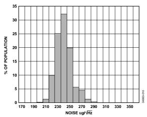
Figure 11. X-Axis Noise Density at 25°C
