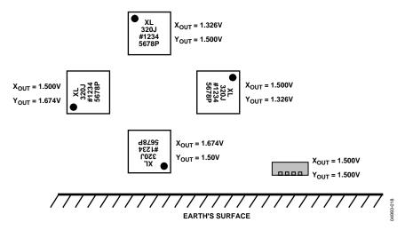
Figure 20. Output Response vs. Orientation
