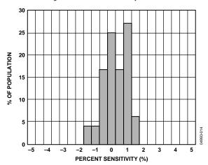
Figure 15. Z vs. Y Cross-Axis Sensitivity
