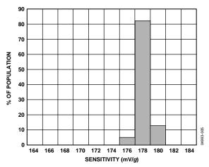
Figure 6. X-Axis Sensitivity at 25°C
