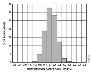
Figure 8. Y-Axis Zero g Bias Temperature Coefficient
