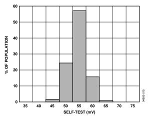
Figure 16. X-Axis Self-Test Response at 25°C
