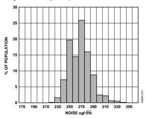
Figure 14. Y-Axis Noise Density at 25°C
