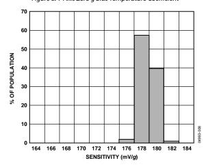
Figure 9. Y-Axis Sensitivity at 25°C
