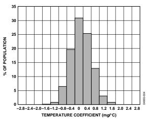
Figure 5. X-Axis Zero g Bias Temperature Coefficient
