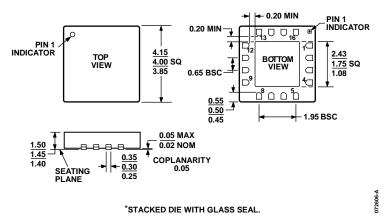
Figure 21. 16-Lead Lead Frame Chip Scale Package [LFCSP\_LQ] 4 mm × 4 mm Body (CP-16-5a\*) Dimensions shown in millimeters
