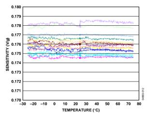
Figure 13. Sensitivity vs. Temperature—Parts Soldered to PCB
