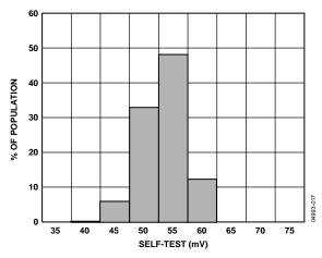
Figure 18. Y-Axis Self-Test Response at 25°C
