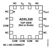
Figure 2. Pin Configuration
